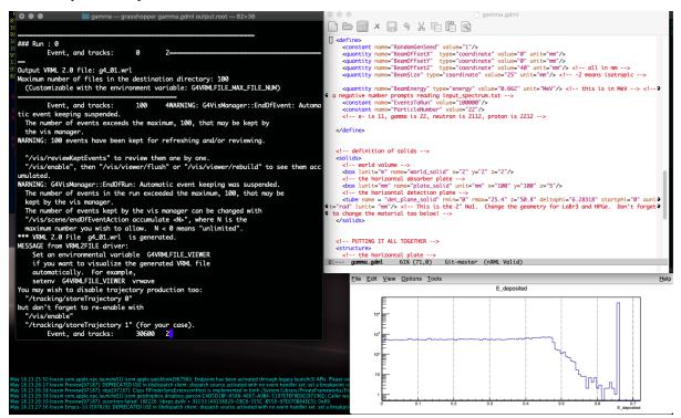
A visualization of a 1 MeV neutron beam entering a water volume, undergoing thermalization.
